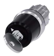
key-operated switch Siemens, 22 mm, round, metal, shiny, lock no. LSG1, with 2 keys, 2 switch positions O-I, latching, actuating angle 90°, 10:30h/13:30h, key removal O+I, with laser labeling, upper case and lower case, always upper case at beginning of line
