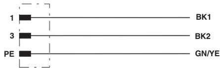
Contact assignment of the M12 plug
