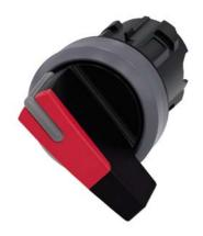
Selector switch, illuminable, 22 mm, round, plastic with metal front ring, red, selector switch, long, 2 switch positions O-I, latching, actuating angle 90°, 10:30h/13:30h, with laser labeling, upper case and lower case, always upper case at the beginning of the word
