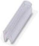
Conductor marker carrier, transparent, unlabeled, Mounting type: slide on, Cable diameter: 6-10 mm, Lettering field: 4 x 15 mm
