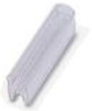
Conductor marker carrier, transparent, unlabeled, Mounting type: slide on, Cable diameter: 2-4 mm, Lettering field: 4 x 15 mm
