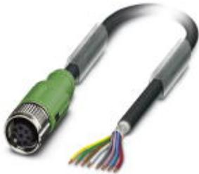
Sensor/Actuator cable, 8-position, PUR halogen-free, black-gray RAL 7021, shielded, free cable end, on Socket straight M12 SPEEDCON, A-coded, Cable length: 5 m
