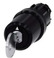
key-operated switch Siemens, 22 mm, round, plastic, lock number SSG10, with 2 keys, 3 switch positions I>O<II, momentary contact on the left, latching on the right, actuating angle 2x45°, 10:30h/12h/13:30h, key removal O+II, with laser labeling, inscription or symbol customer-specific selection with SIRIUS ACT configurator (CIN)
