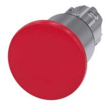
Mushroom pushbutton, 22 mm, round, metal, shiny, red, 40 mm, 3 switch positions, latches after pushing in, unlatches by pull-to-unlatch mechanism to center position, after pulling out the button Retraction to center position, with laser labeling, upper case and lower case, always upper case at the beginning of the word
