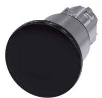
Mushroom pushbutton, 22 mm, round, metal, shiny, black, 40 mm, 3 switch positions, after pushing in Retraction to center position, after pulling out the button Retraction to center position, with laser labeling, inscription or symbol Customer-specific selection with SIRIUS ACT configurator (CIN)
