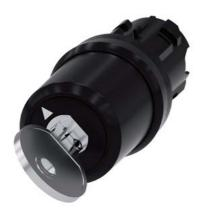
Key-operated switch BKS, 22 mm, round, plastic, lock number S1, with 2 keys, 2 switch positions O-I, latching, actuating angle 90°, 10:30h/13:30h, Key removal O Z=50-unit packaging
