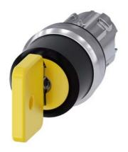
Key-operated switch O.M.R, 22 mm, round, metal, shiny, lock number 73033, yellow, with 2 keys, 3 switch positions I>O<II, momentary contact on the left, latching on the right, actuating angle 2x45°, 10:30h/12h/13:30h, Key removal II, with laser labeling, upper case and lower case, always upper case at the beginning of the word
