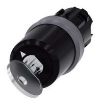
key-operated switch Siemens, 22 mm, round, plastic with metal front ring, lock number SSG10, with 2 keys, 2 switch positions O-I, latching, actuating angle 90°, 10:30h/13:30h, key removal O+I, with laser labeling, lower case
