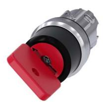
Key-operated switch O.M.R, 22 mm, round, metal, shiny, lock number 73037, red, with 2 keys, 2 switch positions O-I, latching, actuating angle 90°, 10:30h/13:30h, key removal O+I, with laser labeling, upper case and lower case, always upper case at beginning of line
