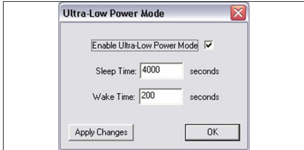
FIGURE 2-9: CSACdemo Ultra-Low Power Mode Configuration Panel.
