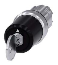
Key-operated switch BKS, 22 mm, round, metal, shiny, lock number S1, with 2 keys, 3 switch positions I-O-II, latching, actuating angle 2x45°, 10:30h/12h/13:30h, Key removal I+O+II, with laser labeling, upper case and lower case, always upper case at beginning of line
