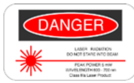
Figure 5. Warning logotype label for Class IIIa lasers.
