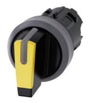
Selector switch, illuminable, 22 mm, round, plastic with metal front ring, yellow, selector switch, short, 3 switch positions I>O<II, momentary contact on the left, latching on the right, actuating angle 2x45°, 10:30h/12h/13:30h, with laser labeling, upper case and lower case, always upper case at the beginning of the word
