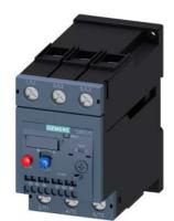
Overload relay 22...32 A Thermal For motor protection Size S2, Class 10 Stand-alone installation Main circuit: Screw Auxiliary circuit: spring-type terminal Manual-Automatic-Reset
