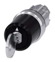
key-operated switch Siemens, 22 mm, round, metal, shiny, lock number SSG10, with 2 keys, 3 switch positions I-O-II, latching, actuating angle  $2x45^{\circ},\,10:30h/12h/13:30h,$  key removal I+O+II, with laser labeling, upper case and lower case, always upper case at the beginning of the word
