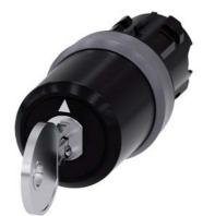
key-operated switch Siemens, 22 mm, round, plastic with metal front ring, lock number SSG10, with 2 keys, 3 switch positions I-O-II, latching, actuating angle  $2x45^{\circ}$ , 10:30h/12h/13:30h, key removal O+I, with laser labeling, upper case and lower case, always upper case at the beginning of the word
