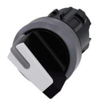
Selector switch, illuminable, 22 mm, round, plastic with metal front ring, white, selector switch, short, 2 switch positions O<I, momentary contact type, Actuating angle 45°, 10:30h/12h, with laser labeling, inscription or symbol Customer-specific selection with SIRIUS ACT configurator (CIN)
