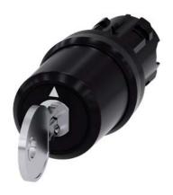
key-operated switch Siemens, 22 mm, round, plastic, lock number SSG10, with 2 keys, 3 switch positions I-O-II, latching, actuating angle  $2x45^{\circ}$ , 10:30h/12h/13:30h, key removal II, with laser labeling, upper case
