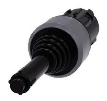
Coordinate switch, 22 mm, round, plastic with metal front ring, black, 4 switch positions, latching, with mechanical interlocking, with laser labeling, lower case
