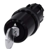
Key-operated switch BKS, 22 mm, round, plastic, Lock No. E9 (VW), without key, 3 switch positions I-O-II, latching, actuating angle 2x45°, 10:30h/12h/13:30h, Key removal I+O+II, with laser labeling, upper case and lower case, always upper case at the beginning of the word
