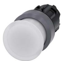
Illuminated mushroom pushbutton, 22 mm, round, plastic with metal front ring, white, 30 mm, momentary contact type, with laser labeling, upper case and lower case, always upper case at the beginning of the word
