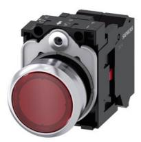
Illuminated pushbutton, 22 mm, round, Metal, shiny, red, pushbutton, flat, momentary contact type, with holder, 1 NC, LED module with integrated LED 230 V AC, spring-type terminal, with laser labeling, upper case
