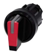
Selector switch, illuminable, 22 mm, round, plastic, red, selector switch, short, 3 switch positions I>O<II, momentary contact type, actuating angle  $2x45^{\circ}$ , 10:30h/12h/13:30h Z=50-unit packaging
