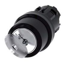
RONIS key-operated switch, 22 mm, round, plastic, lock number 455, with 2 keys, 2 switch positions O<I, momentary contact type, Actuating angle 45°, 10:30h/12h, key removal O, with laser labeling, upper case and lower case, always upper case at the beginning of the word
