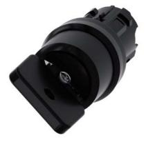
Key-operated switch O.M.R, 22 mm, round, plastic, lock number 73034, black, with 2 keys, 2 switch positions O-I, latching, actuating angle 90°, 10:30h/13:30h, Key removal O+I Z=50-unit packaging
