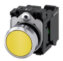
Pushbutton, 22 mm, round, metal, shiny, yellow, pushbutton, flat, momentary contact type, 1 NO, spring-type terminal, with laser labeling, symbol number according to, ISO 7000 or IEC 60417
