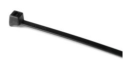
High impact and heat stabilized cable ties contain an impact modifier allowing greater flexibility and greater resistance to vibration. Head design contains clamping rails to provide full circumferential compression around bundles.
