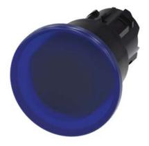
Illuminated mushroom pushbutton, 22 mm, round, plastic, blue, 40mm, latching, pull-to-unlatch mechanism, with laser labeling, symbol number according to, ISO 7000 or IEC 60417
