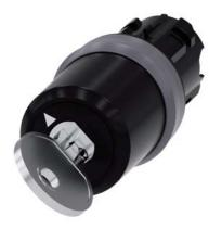
key-operated switch Siemens, 22 mm, round, plastic with metal front ring, lock no. LSG1, with 2 keys, 2 switch positions O-I, latching, actuating angle  $90^{\circ}$ , 10:30h/13:30h, key removal O, Z=50-unit packaging
