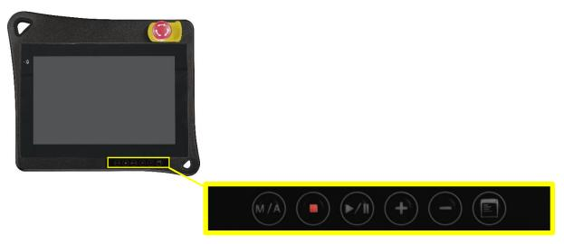
The TP 100-1's membrane keys are located at the lower-right of the teach pendant, each membrane key is mapping to the real-keyboard signal, review the key definitions below:
