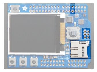
The micro SD card slot can be used to read/write data from any micro SD card using the Arduino libraries. The SD card is connected to the SPI pins as well as Digital #4 for Chip Select
