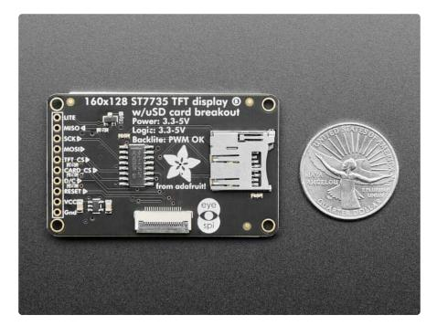
This display breakout comes with an EYESPI connector! This 18-pin 0.5mm pitch FPC connector has a flip-top connector for using a flex cable to hook up your display. It
