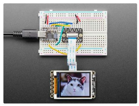
This display now comes with an EYESPI connector. This connector allows you to connect your display without soldering. There are <u>EYESPI cables</u> () available in multiple lengths, which means you can find one to fit any project. This is especially useful if your project requires the display to be freestanding, and not tied directly into a breadboard. Inspired by the popularity of STEMMA QT, it provides plug-n-play for displays!
