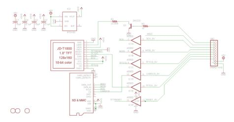
For the level shifter we use the CD74HC4050 which has a typical propagation delay of  $^{\sim}10\text{ns}$
