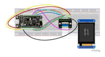
breakout Vin to Feather 3.3V (red wire) breakout Lite to Feather 3.3V (yellow wire) breakout Gnd to Feather GND (black wire) breakout SCK to Feather SCK (grey wire) breakout MISO to Feather MI (green wire) breakout MOSI to Feather MO (purple wire)
