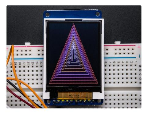
Once uploaded, the Arduino should perform all the test display procedures! If you're not seeing anything - first check if you have the backlight on, if the backlight is not lit
