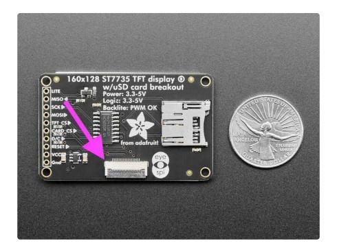
The EYESPI cables are 18 pin 0.5mm pitch flex cables. They are ~9.6mm wide, and designed to fit perfectly into the EYESPI connector. Adafruit currently offers EYESPI cables in three different lengths: 50mm (), 100mm (), and 200mm ().
