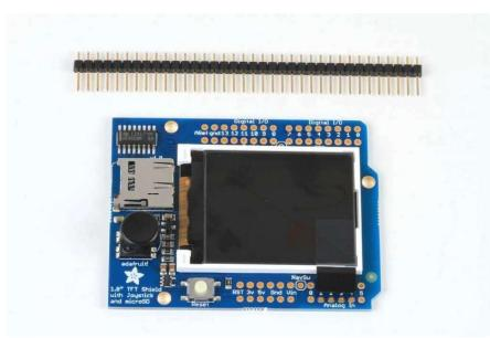
The shield comes with all surface mount parts pre-soldered. All that remains is to install the headers!
