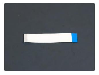
Each EYESPI cable has blue stripes on either end. On the other side of the cable, underneath the blue stripe, are the connector pins that make contact with the FPC connector pins on the display or breakout.
