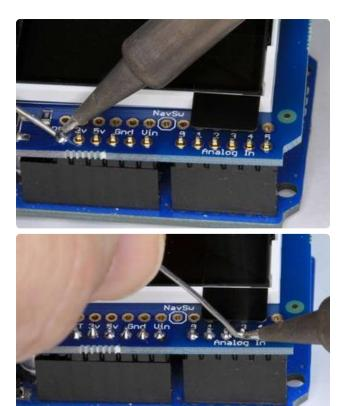
And Solder! Solder each pin to assure good electrical contact.
