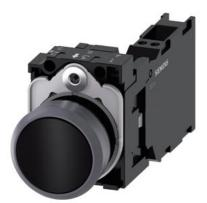
Pushbutton, 22 mm, round, plastic with metal front ring, black, pushbutton, flat, momentary contact type, with holder, 1 NO+1 NC, spring-type terminal, with laser labeling, upper case and lower case, always upper case at the beginning of the word
