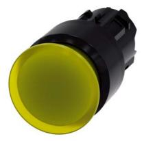
Illuminated mushroom pushbutton, 22 mm, round, plastic, yellow, 30 mm, latching, pull-to-unlatch mechanism, with laser labeling, inscription or symbol Customer-specific selection with SIRIUS ACT configurator (CIN)
