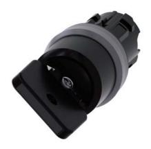
Key-operated switch O.M.R, 22 mm, round, plastic with metal front ring, lock number 73034, black, with 2 keys, 2 switch positions O-I, latching, actuating angle 90°, 10:30h/13:30h, key removal O+I, with laser labeling, inscription or symbol Customer-specific selection with SIRIUS ACT configurator (CIN)
