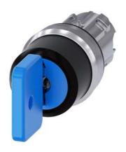
Key-operated switch O.M.R, 22 mm, round, metal, shiny, lock number 73038, blue, with 2 keys, 3 switch positions I-O-II, latching, actuating angle 2x45°, 10:30h/12h/13:30h, Key removal I+O+II, with laser labeling, upper case and lower case, always upper case at the beginning of the word
