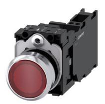
Illuminated pushbutton, 22 mm, round, metal, shiny, red, pushbutton, flat, momentary contact type, with holder, 1 NO+1 NC, LED module with integrated LED 24 V AC/DC, spring-type terminal, with laser labeling, upper case
