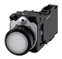
Illuminated pushbutton, 22 mm, round, plastic, white, pushbutton, flat, momentary contact type, with holder, 1 NO+1 NC, LED module with integrated LED 24 V AC/DC, screw terminal, Z=20-unit packaging
