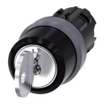
RONIS key-operated switch, 22 mm, round, plastic with metal front ring, lock number SB30, with 2 keys, 3 switch positions I-O-II, latching, actuating angle 2x45°, 10:30h/12h/13:30h, Key removal II, possible special locks: SB31, 421, 455, with laser labeling, upper case and lower case, always upper case at the beginning of the word
