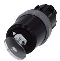
Key-operated switch BKS, 22 mm, round, plastic with metal front ring, Lock No. E2 (VW), without key, 2 switch positions O-I, latching, actuating angle  $90^{\circ}$ , 10:30h/13:30h, key removal O+I, with laser labeling, lower case
