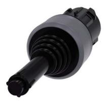
Coordinate switch, 22 mm, round, plastic with metal front ring, black, 4 switch positions, momentary contact type, with mechanical interlocking, with laser labeling, upper case
