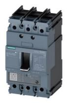
circuit breaker 3VA5 UL frame 125 3-pole, starter protection TM120M, AM, In=10A without overload protection short-circuit protection li=5...12 x In nut keeper kit on both sides
