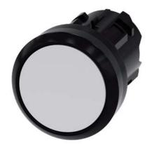
Pushbutton, 22 mm, round, plastic, white, pushbutton, flat, latching, Pushto-release mechanism, with laser labeling, inscription or symbol Customer-specific selection with SIRIUS ACT configurator (CIN)
