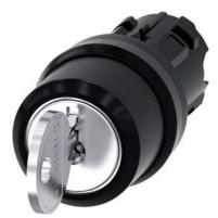
RONIS key-operated switch, 22 mm, round, plastic, lock number SB30, with 2 keys, 3 switch positions I-O<II, left latching, right momentary contact type, actuating angle  $2x45^{\circ}$ , 10:30h/12h/13:30h, key removal O+I, possible special locks: SB31, 421, 455 Z=50-unit packaging
