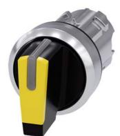
Selector switch, illuminable, 22 mm, round, metal, shiny, yellow, selector switch, short, 3 switch positions I>O<II, momentary contact type, actuating angle 2x45°, 10:30h/12h/13:30h, Z=50-unit packaging
