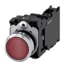
Illuminated pushbutton, 22 mm, round, Metal, shiny, red, pushbutton, flat, momentary contact type, with holder, 1 NO+1 NC, LED module with integrated LED 230 V AC, spring-type terminal, with laser labeling, upper case and lower case, always upper case at the beginning of the word
