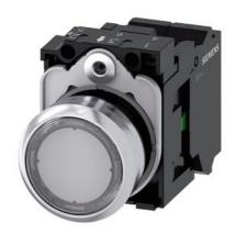
Illuminated pushbutton, 22 mm, round, metal, shiny, transparent, pushbutton, flat, momentary contact type, with holder, 1NO, LED module with integrated LED 230 V AC, spring-type terminal, Z=20-unit packaging
