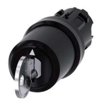
Key-operated switch IKON, 22 mm, round, plastic, lock number 360012K1, with 2 keys, 3 switch positions I-O-II, latching, actuating angle 2x45°, 10:30h/12h/13:30h, Key removal I+O+II, with laser labeling, upper case and lower case, always upper case at the beginning of the word
