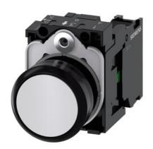
Pushbutton, 22 mm, round, plastic, white, pushbutton, flat, momentary contact type, with holder 1 NO, screw terminal, with laser labeling, symbol number according to, ISO 7000 or IEC 60417
